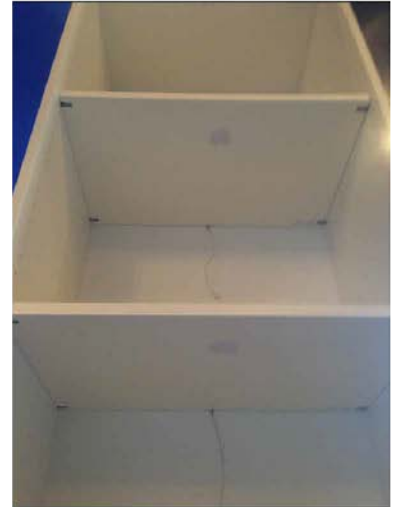
3) Shelves and Wires in place with double sided sticky for LED lights
